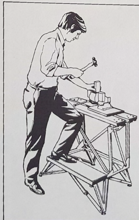
A metalworking vice can be used with the Workmate — simply mount it on a wooden board, screwed to a batten, and clamp the batten between the vice bars.
