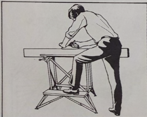
Accurate planing of wood, especially long planks, is easy with the massive vice bars.
