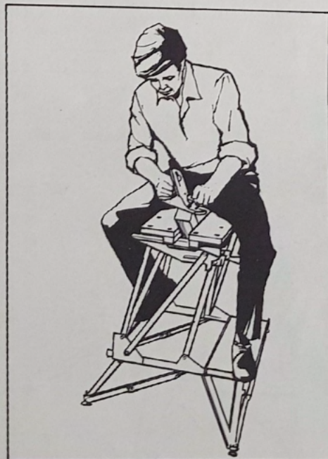
The massive vice bars hold the work piece securely for shaping, forming, sanding etc.
