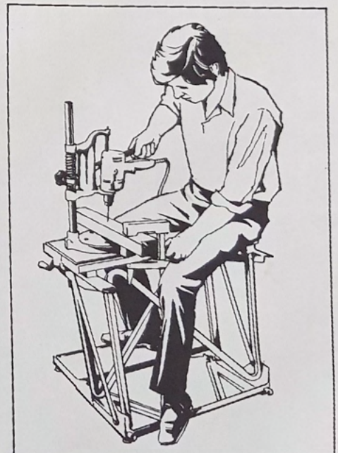
Power tools such as a circular saw, vertical drill stand, woodworking lathe, can be clamped within the vice jaws using a wooden board screwed to a batten.
