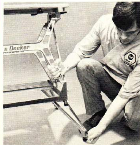
6. To maintain a rigid and balanced Workmate in the "workbench" position, adjust the extension leg screw feet in the same manner as in "sawhorse" position.
