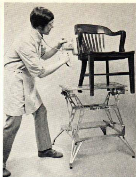
13. The Workmate brings the job up to where you can reach and see it, conveniently, even with hard-to-hold items.
