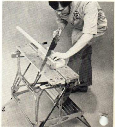
6. Holding a mitre box for more accurate angle cuts. Note: For added rigidity, exert your body weight on the Workmate's base board when sawing or performing other tasks.
