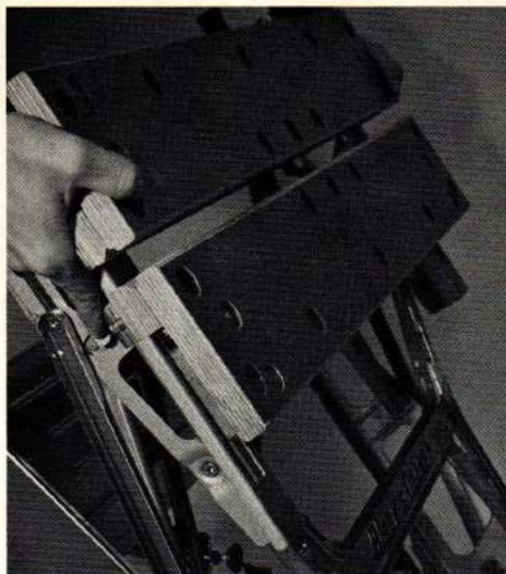
1. Press the two release buttons located, as shown, on either side of the Workmate.
