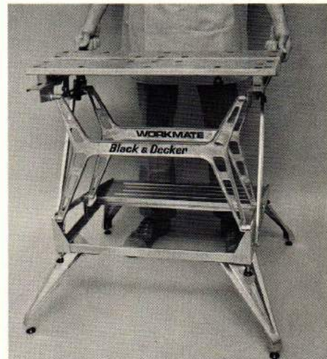
5. Always make sure that each leg into its extended position. Ensure adjustable feet for "sawhorse" position do not prevent the legs from fully locking. This will ensure the safe use of the Workmate at this upper working height.
