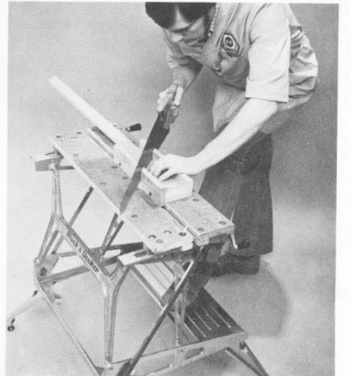
6. Holding a mitre box for more accurate angle cuts. Note: For added rigidity, exert your body weight on the Workmate's base board when sawing or performing other tasks.
