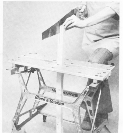
5. Gripping hard-to-hold objects while sawing.
