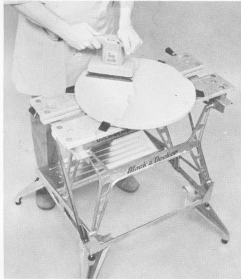
11. Power sand the most irregular shapes and use exactly the pressure that's needed. There are no sudden surprises when the item holds still.
