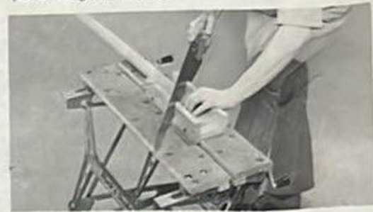
6. Holding a mitre box for more accurate angle cuts. Note: For added rigidity, exert your body weight on the Workmate's base board when sawing or performing other tasks.
