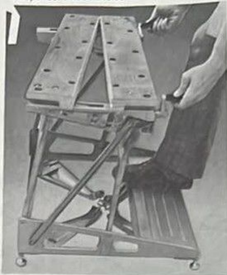
2. Tapering the vise opening using the independent vise handles.
