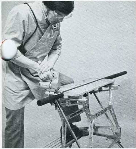
7. Sawing tubular pieces is easy when they are held horizontally in the specially designed V-grooves running along the face of the vise jaws.
