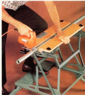
V-grooves grip tubular objects.
