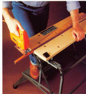
V-grooves grip tubular objects.
