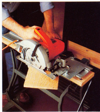
MITREMATE™ Saw Guide attachment adds accuracy to cuts.
