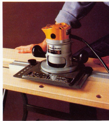
ROUTERMATE™ Shaping Guide attachment makes routing easier.
