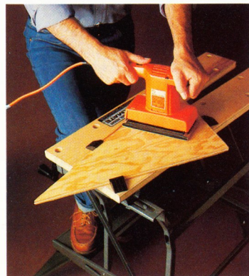
Pegs hold irregular and circular objects.
