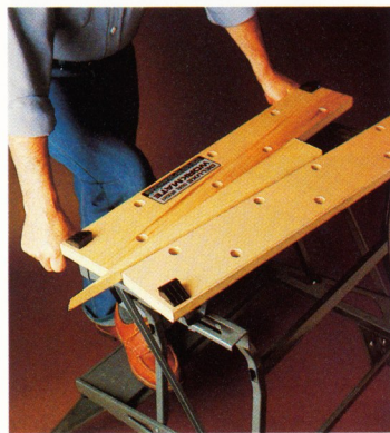
Vise jaws adjust to take wedge shapes.
