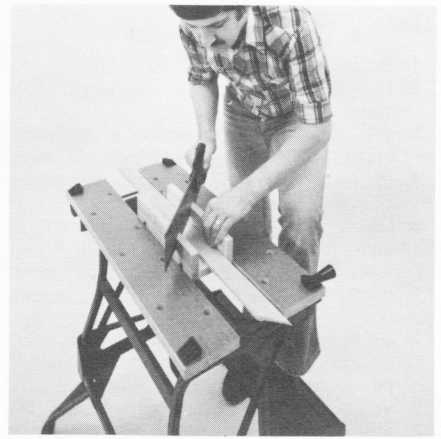
6. Holds a mitre box for more accurate angle cuts. Note: Place foot on WORKMATE step for added rigidity.
