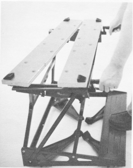
2. Tapering the vise opening, using the independently operated vise handles.
