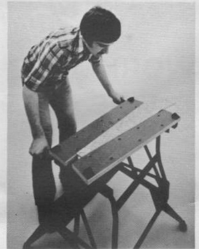
5. Because each end of the vise works independently of the other, tapered objects can be held securely.
