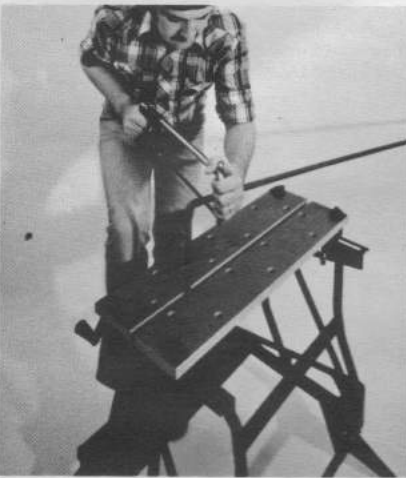
8. Vertical V-grooves in the face of the vise jaws permit rigid vertical grasping of tubular objects.
