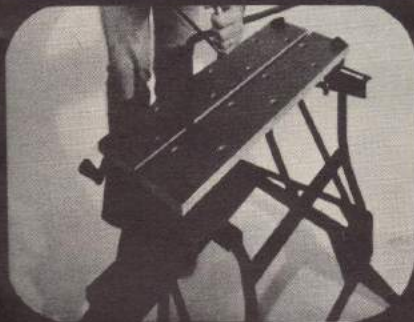
V-grooves hold pipe and tubing up to 5 1 / 4 " wide.
