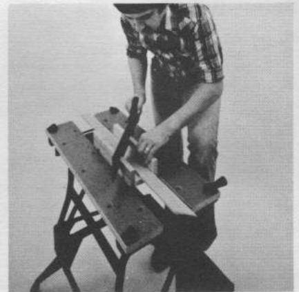
6. Holds a mitre box for more accurate angle cuts. Note: Place foot on Work Center step for added rigidity.
