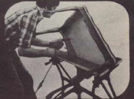
Independent vise jaws allow clamping of irregularly shaped or tapered objects: bikes, furniture, doors, shutters, etc.
