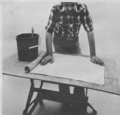
1. When the project calls for extra work space, you can make a work table by attaching a block of wood to the underside of a piece of plywood. Makes an extra long table surface for a work or play occasion. Center table over center of vise jaws.
