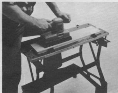
11. Power sand the most irregular shapes. Swivel grips hold material securely.
