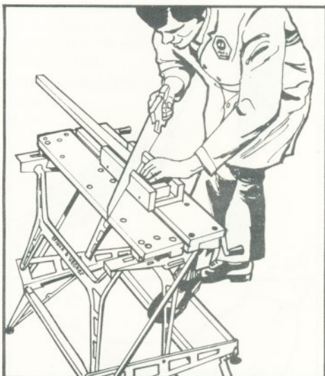
6. Holding a mitre box for more accurate angle cuts. Note: for added rigidity, exert your body weight on the Workmate's base board when sawing or performing other tasks.
